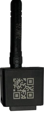
The Core is the brain and transmitter of any meter that it connects to. The Core can be swapped between various devices built to measure utilities such as electricity, water and gas.
